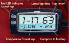
The transmitter sends an invisible infra-red (IR) beam across the track. As your car passes thru the beam the receiver records the lap time and shows it on the display instantly. Try different lines to get the best lap times possible.
