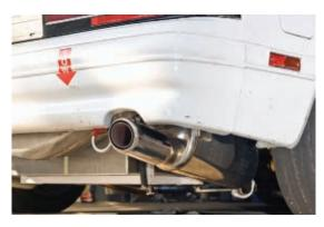
(ABOVE) We opted for Racing Beat's dual exhaust, which flows well while keeping the sound from the rotary tolerable. (BELOW) Engine management in Super Touring is open, so use of systems like Electromotive's TEC-GT is legal.
