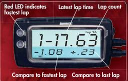
A transmitter sends an invisible infra-red (IR) beam across the track. As your car passes thru the beam the receiver records the lap time and shows it on the display instantly. Try different lines to get the best lap times
