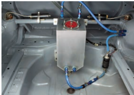
(LEFT) The brake and suspension package on this BMW has already proven its worth, but planned improvements could result in even quicker Solo runs. (ABOVE) The tiny 3-gallon fuel cell means there is minimal unnecessary weight in the trunk.
