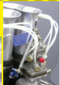
Lucas MKII Metering Unit on Kinsler manifold
