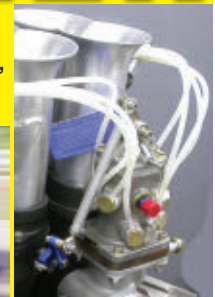
Lucas MKII Metering Unit on Kinsler manifold
