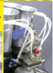
Lucas MKII Metering Unit on Kinsler manifold
