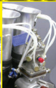
Lucas MKII Metering Unit on Kinsler manifold
