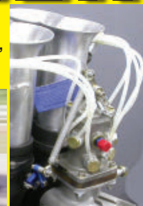
Lucas MKII Metering Unit on Kinsler manifold
