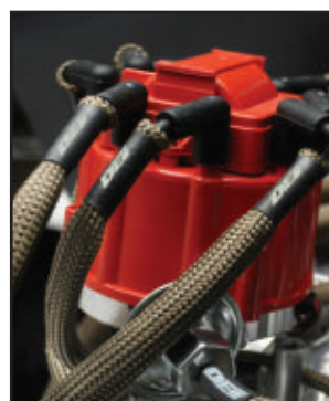
Protection for spark plug wires to prevent burning and cracking
