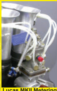
Lucas MKII Metering Unit on Kinsler manifold
