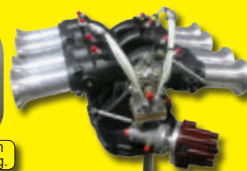
Super Vette, Riley Tube chassis, engines by Lee Muir. Ran Kinsler crossram manifold and Lucas mechanical metering.
