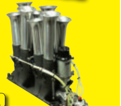
1971 McLaren M8F Can Am car. Ran Kinsler prepared MacKay intake Manifold with Lucas mechanical metering.
